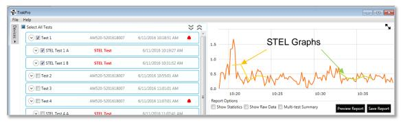
Also, when STEL tests are selected and displayed on the Graph, the scrolling graphing analysis function which displays the time / date stamp, also shows both data points at any high or low point of the STEL data as shown below.
