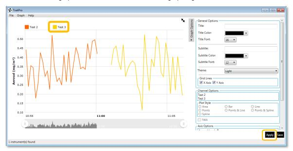
In the example below, the data graph for Test 3 has been closed and only Test 2 is displayed.
